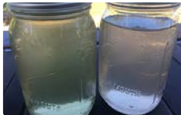
Before and after — produced-water jar samples treated with DZ 9450.
