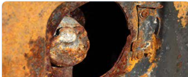
UNDER-DEPOSIT CORROSION IS HALTED ONCE BIOFILM IS REMOVED.
